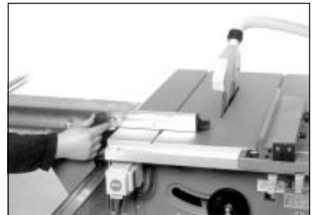
Set fence extrusion closely against the blade, tighten star knobs.
